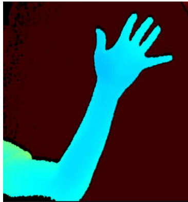
Figure 24 Depth map of a hand showing that the high resolution of the depth camera generates distinctly separated fingers.
