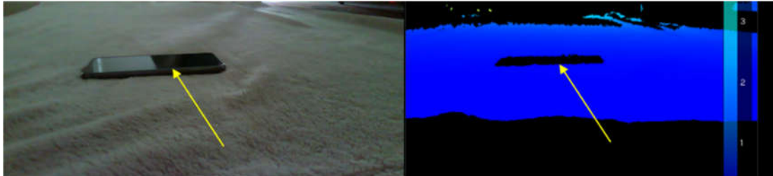
Figure 18 When the light is incident upon a smooth surface at low angles, there will be no reflected light back into the receiver. The light bounces off the phone surface without ever coming back into the photodiode.
