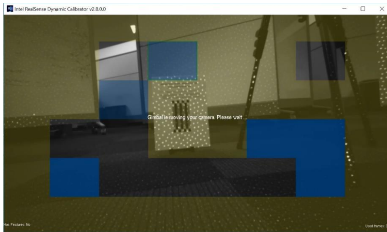
Figure 5-3 Hybrid Dynamic Calibration – Target-less Phase
