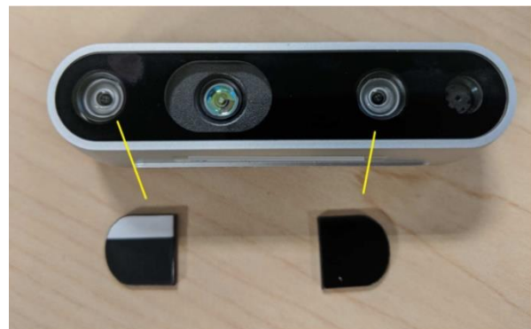
Figure 22 IR pass filters ready to be attached to D435/D435i
