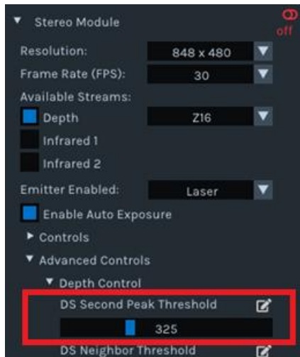
Figure 3 DS Second Peak Threshold control in RS Viewer
