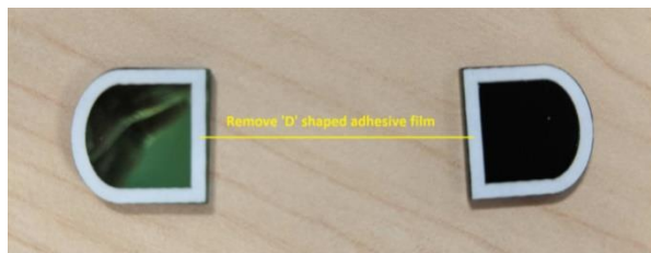
Figure 21 Pre-cut double-sided adhesives attached to the IR pass filter
