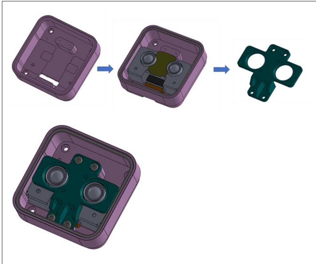
Figure 7-15. Stereo Depth Module Mid-Mounting – D401
