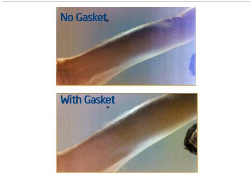
Figure 7-9. Example of Light Leakage Effects
