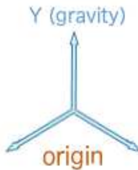
Fig. 4c. The origin coordinate system for T265.
