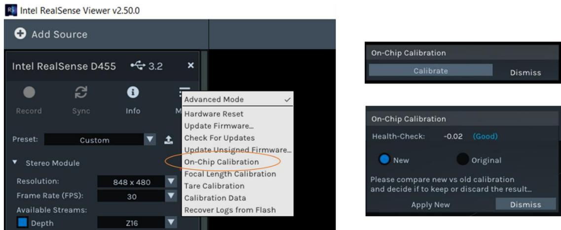
Figure 7. The on-chip self-calibration functions can be accessed in the Intel RealSense Viewer app. Once the calibration routine has been run, it will provide the result of Health-Check and ability to toggle between old and new calibration table. “Apply New” will burn it to flash on the camera and “Dismiss” will cancel the operation and keep the original calibration.
