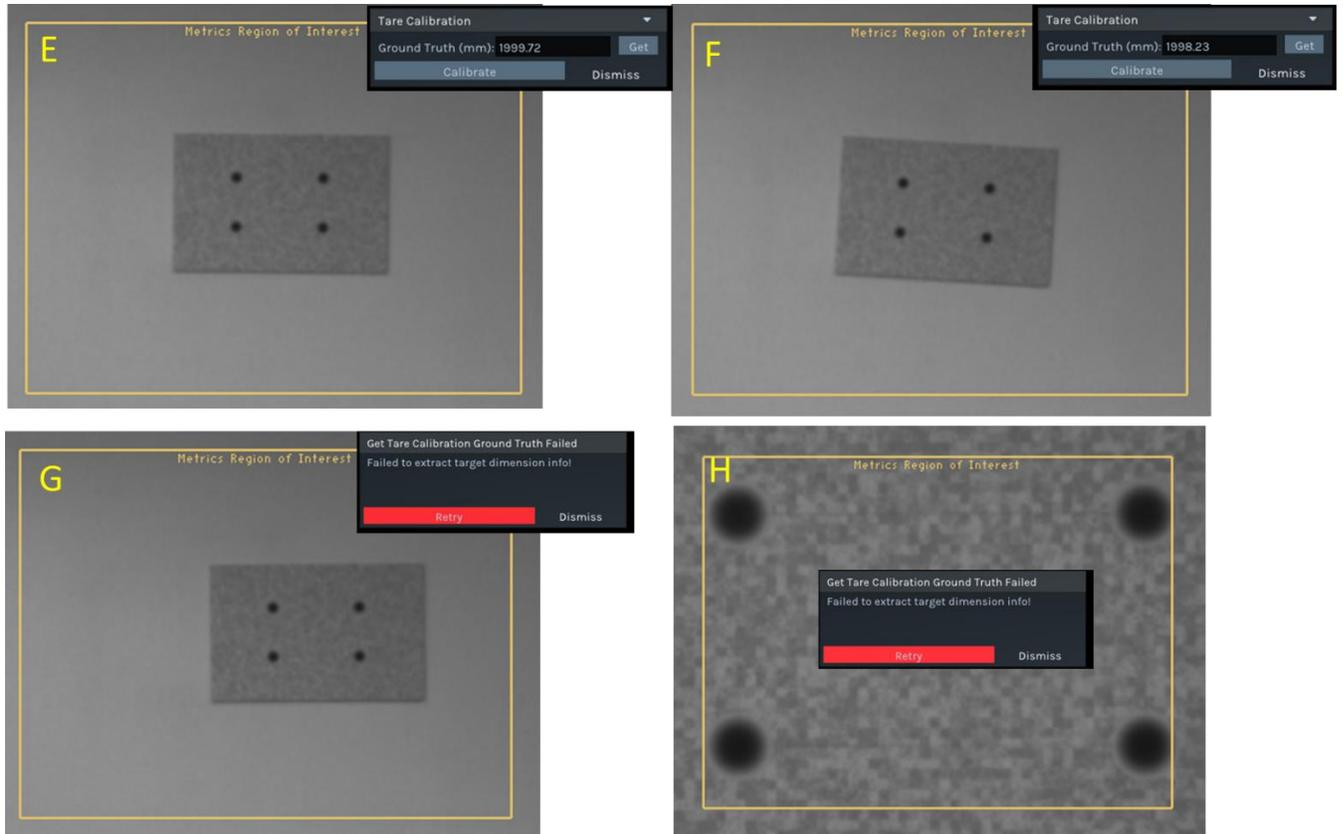
**Figure A4.** Examples of various target alignments with a D435. A-C: consistent and accurate results (within 2mm) for off-center and slightly rotated target at 1000mm. D: target is too far from center of ROI resulting in error message. E-F: examples of acceptable alignment at 2000mm (error < 2mm). G: target too far from center resulting in error message. H: Target centered but too close (400mm) resulting in error message due to spots too close to ROI border.
