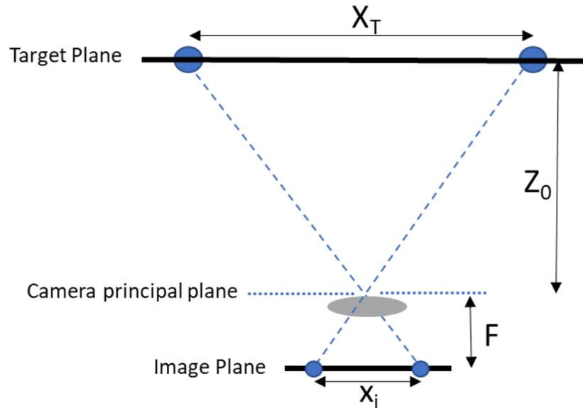
**Figure A2. Principle of operation for GT measurement using two markers. GT ( $Z_0$ ) can be calculated from the known target size ( $X_T$ ), camera focal length ( $F$ ), and the measured image size of the target ( $x_i$ ). The concept can be easily generalized to any larger number of markers.**
