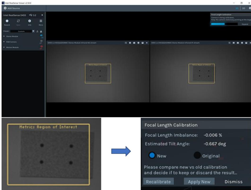
Figure B4. Slight rotation of target about Z axis is acceptable. The Left camera image and corresponding successful FL measurement is shown.
