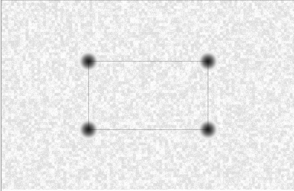
**Figure A1. Example of target used for GT measurement. The markers are Gaussian blurs forming the vertices of a rectangle. The background is a low contrast texture which provides sufficient texture for on-chip and tare calibration. This target is designed with marker separations of 175mm in X and 100mm in Y, marker diameter of 30mm, and to be printed onto an 11x17" format. See Appendix A for other formats and printing instructions.**
