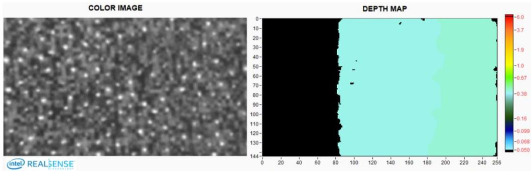
Figure 4. Example zoomed-in 256x144 image of a D435 monochrome image (from left imager) and depth map, as observed by looking at a textured target mounted on a flat wall. The black bar on the left is expected and acceptable. In general, it is important to have >35% of the depth map show depth values (non-zero). In this example the IR projector was left on, but we recommend turning it off when pointing at a well-textured scene.
