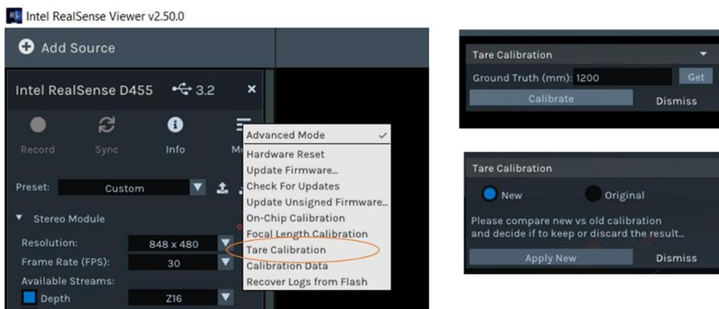
Figure 10. The tare functions can be accessed in the Intel RealSense Viewer app. A ground truth value needs to be entered, or use Get option which will be explained in next section.
