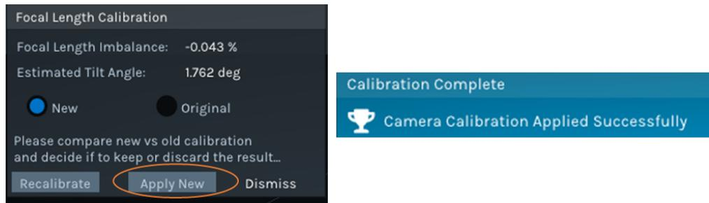
**Figure B3. Sample focal length calibration result. The reported focal length imbalance is the corrected ratio for the measured set-up horizontal tilt angle. If “Apply New” is selected, a “Calibration Complete” message is displayed indicating successful updating of focal length values.**
