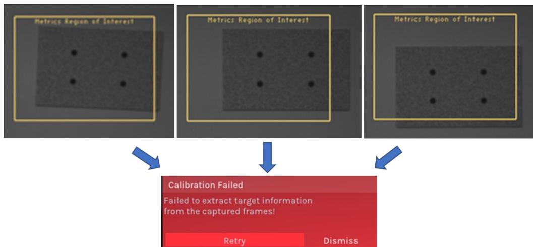
Figure B5. Examples of unacceptable target alignment. The Left camera image is shown for excessive Z-rotation (Left), target shifted too far right (Center), and target shifted too far down (Right). The corresponding error message is shown below.
