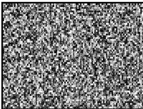
Figure 3. Example A4-sized target with texture which is particularly well suited for both on-chip calibration and depth quality characterization. The exact nature of the texture is not critical, as long as it is semi-random and fairly “noisy” with high spatial frequencies.
