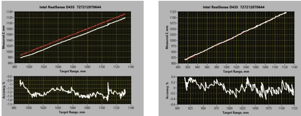
Figure 8. The measured distance vs ground truth (aka target depth). LEFT shows a calibration with a BIAS of -1.2% near 1m distance. RIGHT shows the corrected calibration where the absolute accuracy is mostly limited by the noise of the measurement.
