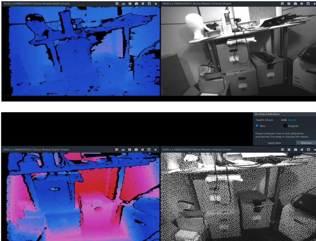
Figure 12. A scenario where on-chip calibration may result in a bad calibration. A scene with variable texture, projector off, and where camera or scene is moving while on-chip calibration is run (top) can lead to an incorrect health-check error and degraded depth. If on-chip calibration is run in a similar manner but with projector on, providing stable texture, then a more accurate health-check number will be returned, and optimal performance is obtained (bottom).
